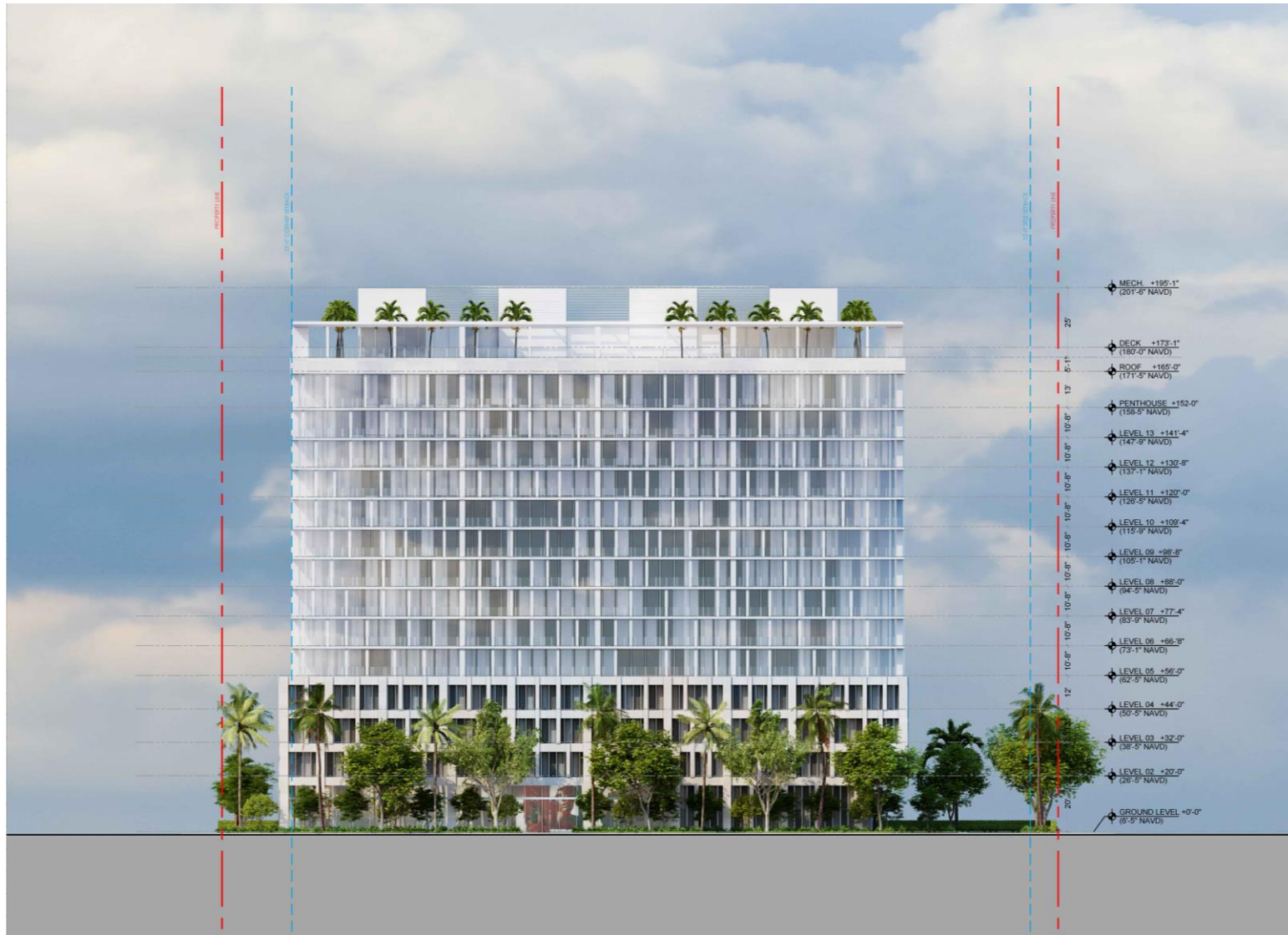
Original Design Presented to CBA in February 2024 15-stories / 180' with conditional use height and yard modifications blocked view corridors
